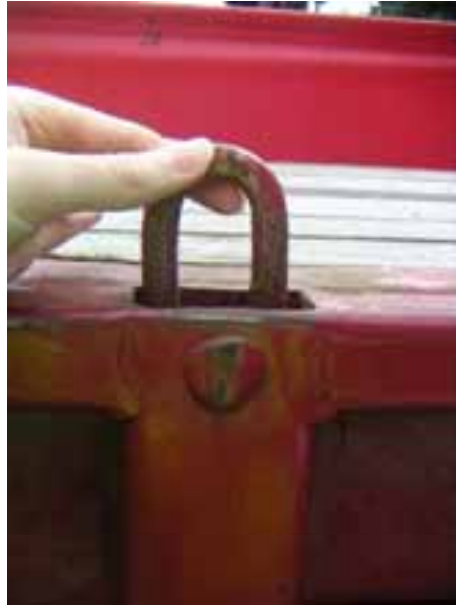
Figure 10 - Retracting fixing eye to avoid trip hazard
