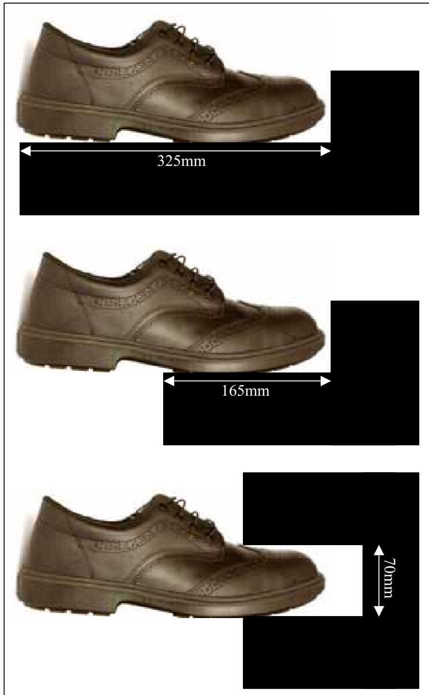
Figure 2 - Schematic of shoe contact area on steps
